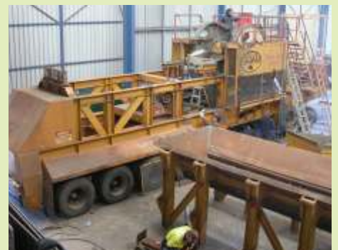
Irvine Engineering's tradesmen rebuild a crusher
