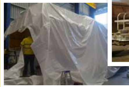
This cone crusher was completely stripped, steam cleaned and painted prior to being shrink wrapped for transport to Barrow Island.
