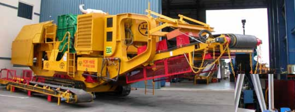
Mobile track mounted impact crusher ready for shrink wrapping
