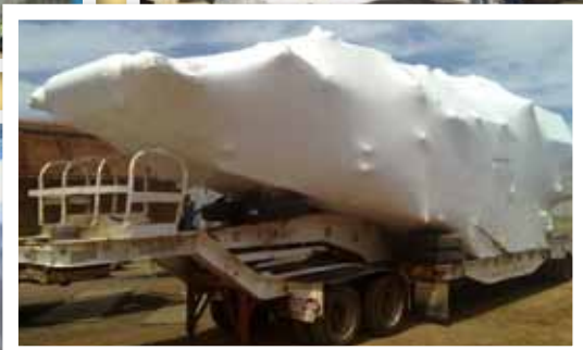
This cone crusher was completely stripped, steam cleaned and painted prior to being shrink wrapped for transport to Barrow Island.
