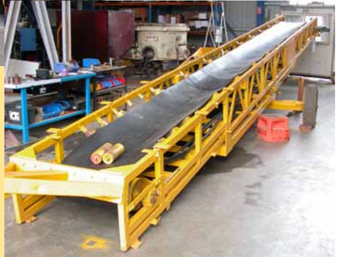
Conveyor being refurbished
